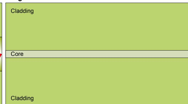
The fibre core comprises of a core and a cladding. This cladding is then covered by a primary coating.
