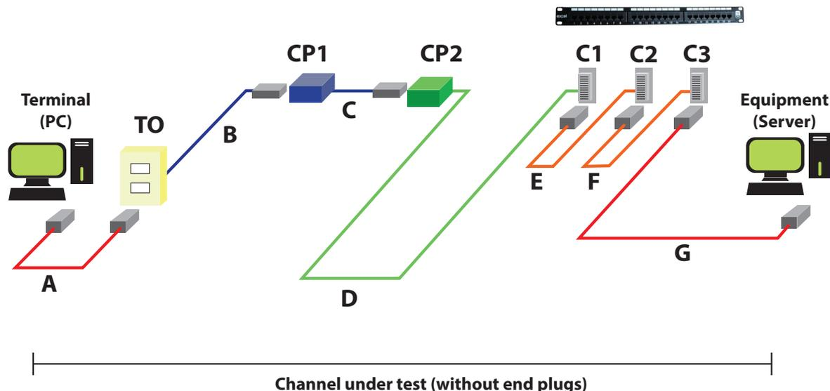
To achieve a 6-connector channel while ignoring the equipment connections you would need to have three patch panels and two consolidation points. Whilst I can understand that there might be a rare occurrence where you may have to link to another building using a short run of the external cable, thereby needing two consolidation points or possibly a localised patching field within a data centre as well as the main patching field, it would still only normally result in a 5-connector channel.
