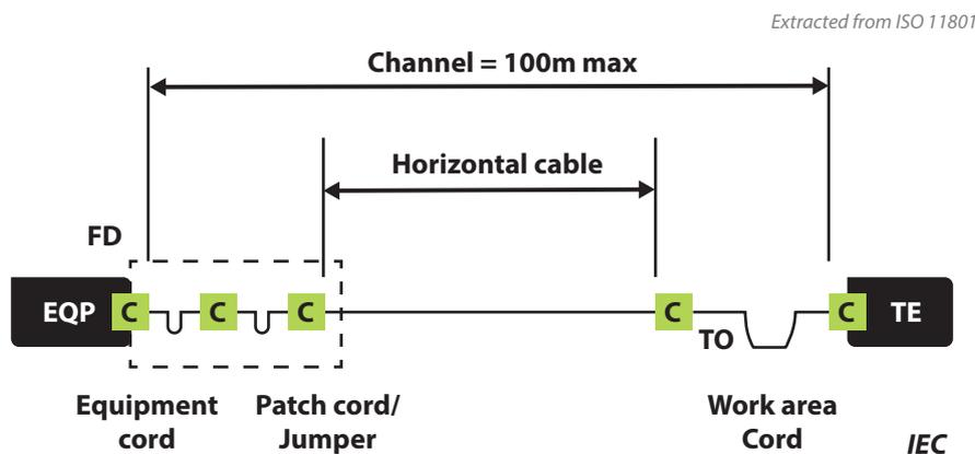
*This model has two patch panels at the equipment end and has three connections*
